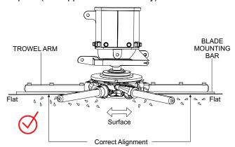
Figure 35. Correct Spider Plate Alignment
